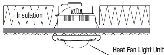
a) Be of a type that can maintain its dimensions and structural integrity when exposed to the maximum surface temperatures of the Heat Fan Light Unit, being 150°C. Refer Specifications above for Insulation classification of the model you have purchased.
