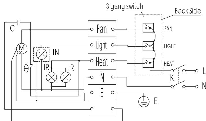
M:Motor C:Capacitor IR:Heat lamp IN:Light lamp
