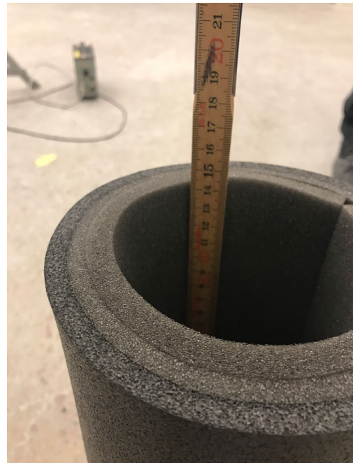
Picture 4 – The inner foam ring started 15 cm into the wall measured from the internal side.
