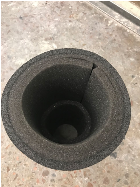
Picture 3 – TL80C dBR with Ø98/81/148 x 200 mm pipe made of polyether foam rings surrounded by PE foam.
