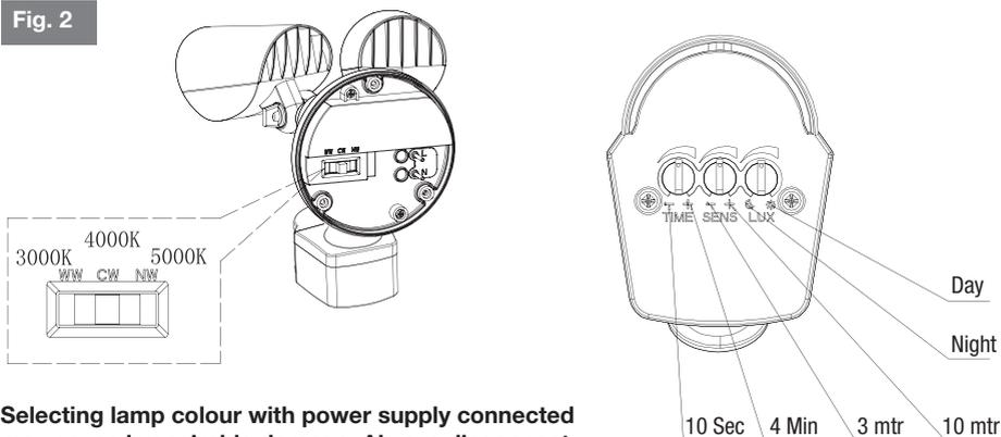
**Selecting lamp colour with power supply connected may cause irreparable damage. Always disconnect at mains before making any colour selection.**
