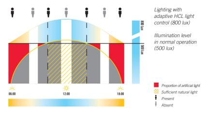
ESYLUX SymbiLogic technology: presence- and daylightdependent adaptive HCL light control.
