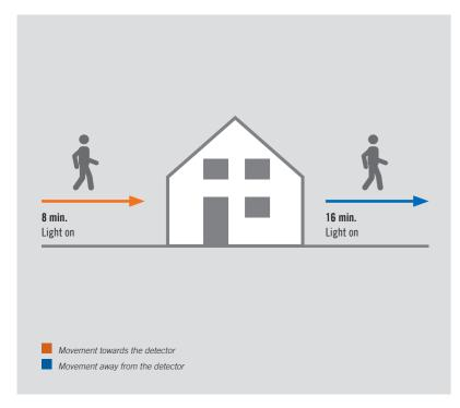
A 230° motion detector is mounted above a door area. If someone enters the house and walks towards the detector, the overrun time ends after an energy-saving 8 minutes. When walking in the opposite direction, the overrun time allows the light to shine for another 16 minutes, thus creating security through an illuminated outdoor area.
