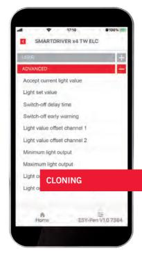
Previously implemented configurations can be stored and transferred to products of the same type via the ESY-Pen using the cloning function.
