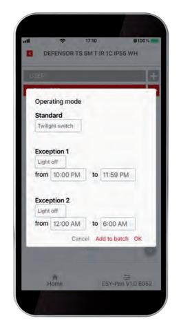
As their name suggests, the DEFENSOR twilight switches switch on the lighting when dusk begins to fall and only switch it off again the next morning once there is sufficient daylight. However, there are various scenarios in which it may be necessary to deviate from this operating mode.
