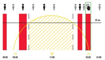
A 200° motion detector is installed on the front of a detached house. In fully automatic mode, it uses motion- and daylight-dependent light control. The user can also switch on the lighting manually from inside using a button.
