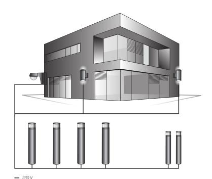
Controlling bollard lights and up-/downlights from the ALVA series using a DEFENSOR motion detector creates a lighting solution for outdoor areas that is every bit as intelligent as it is visually harmonious.
