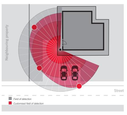
In the example, the maximum field of detection would extend to the street and to the neighbouring property, and as such would result in the lighting frequently being switched on unnecessarily. The range in these zones has therefore been reduced accordingly.
