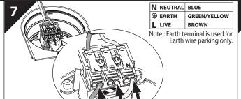
Connect the new/pre-existing cable to the terminal block in accordance with the wiring colours shown.
