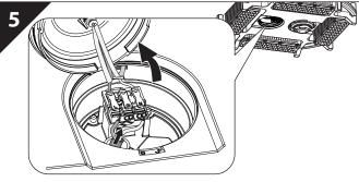
Remove the wiring box cover to expose the connections. Disconnect the wires from the side of the terminal block marked L, & N. Pull the cable through the gland & discard.
