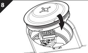
Replace the wiring box cover plate, ensuring no wires are trapped.
