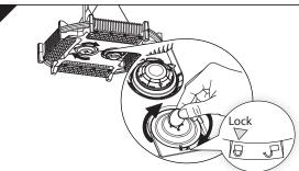
Secure the wiring box cover by rotating in a clockwise direction until the arrow is aligned with the LOCK symbol.
