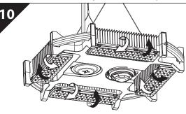
Each LED lightbar can be rotated in/out by up to 30° to adjust the illumination pattern for wide area, aisle, crossroad or T-junction requirements.
