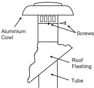
Position the top end of the tube into the cowl.
