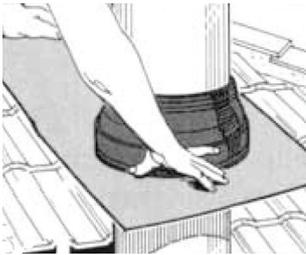
Slide the tile roof flashing down over the tube to the tile roof level. Water can be used as a lubricant.
