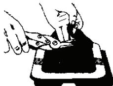
Cut the pliable roof flashing sleeve on the 190/200 marking
