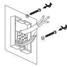
Push the power supply through the cable gland. Affix the rear base to the mounting surface with mounting wall screws supplied. To maintain the IP rating, a round 3 core 0.75mm² (min) cable should be used.
