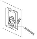
3 Use the rear base to mark the position of screw holes onto the mounting surface. Use a spirit level to ensure correct orientation.
