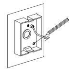
**3** Use the rear base to mark the position of screw holes onto the mounting surface. Use a spirit level to ensure correct orientation.
