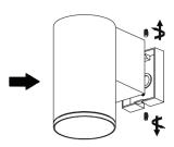
2 Unscrew the fixing cover screws with the allen key supplied and remove the rear mounting base.
