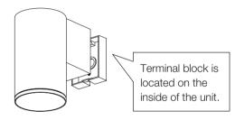
6 Connect the power cables to the terminal block securely using the wiring diagram in Step 7.
