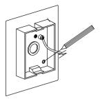
3 Use the rear base to mark the position of screw holes onto the mounting surface. Use a spirit level to ensure correct orientation.
