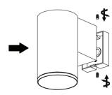
Reattach and screw securely the cover to the base.
