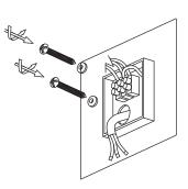
5 Push the power supply through the cable gland. Affix the rear base firmly to the mounting surface with mounting wall screws supplied. To maintain the IP rating, a round 3 core 0.75mm<sup>2</sup> (min) cable should be used.
