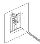
3 Use the rear base to mark the position of screw holes onto the mounting surface. Use a spirit level to ensure correct orientation. Power entry hole should be at the bottom.
