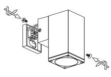
8 Reattach and screw securely the light to the base. Ensure cables are not pinched when closing the unit.
