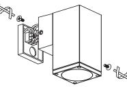
Unscrew the fixing cover screws and remove the rear mounting base.
