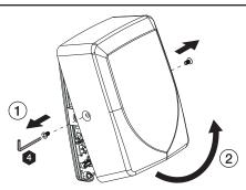
Unscrew front cover from the base of the unit using the hex key provided.
