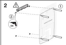
Using the mounting template supplied, mark mounting hole locations for correct height above the floor and drill 4x mounting holes.
