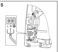
Connect supply and ground wires to terminal block where indicated.
