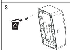
Remove transport screw at the rear of the dryer.
