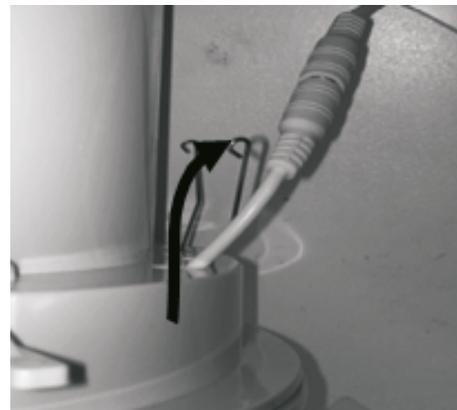
**Note:** LED fascia and LED driver are replaceable. To replace – disconnect female and male connectors and replace new LED fascia or LED driver.
