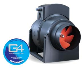
TORPDC100 Designed for G4 Bathrooms ceiling installations on full speed boost mode, with up to 3m duct length, 2 x 90° bends and a soffit mounted fixed louve grille.
